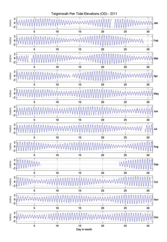
Figure 2: Teignmouth Pier tidal elevations for 2011 relative to Ordnance Datum
