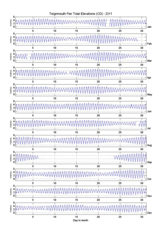
Figure 3: Teignmouth Pier tidal elevations for 2011 relative to Chart Datum
