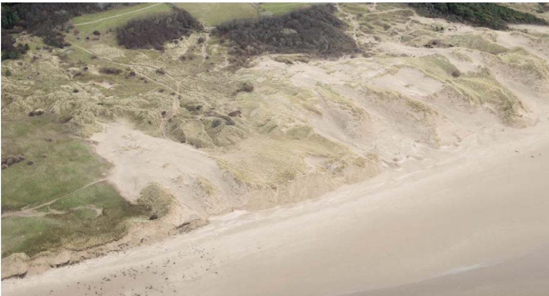
An example of Sefton's oblique photography commissioned as a post-storm survey following the December 5th event. It was flown on the 16th of December and still clearly shows the steep cliffing that has occurred to many of the duned areas and the smoothed, featureless looking beach. The dark dots are blocks of tobacco waste that was buried in the dunes in the 60's and is now being eroded.
